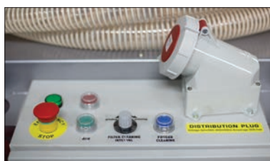
DISTRIBUTION PLUG ON V32-X FOR ATTACHING GRINDER TO THE VACUUM
