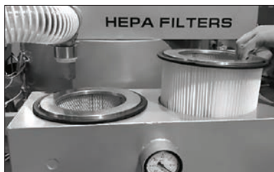
2 HEPA FILTERS, H13 CLASS RATED AT 99.99% AT 0.3 MICRONS
