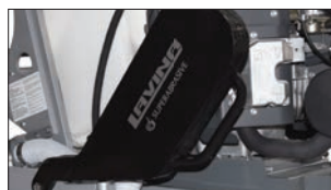
Built-in weights on L32G-X
