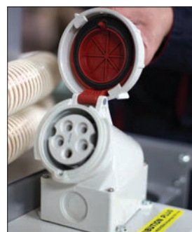
DISTRIBUTION PLUG ON V32-X FOR ATTACHING GRINDER TO THE VACUUM
